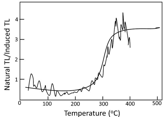
Fig. 3. Plot of the ratio of the natural TL to the ratio of the induced TL as a function of glow curve temperature. The position of the step in the ratio suggests that Sutter's Mill has been heated to approximately 300 °C.
