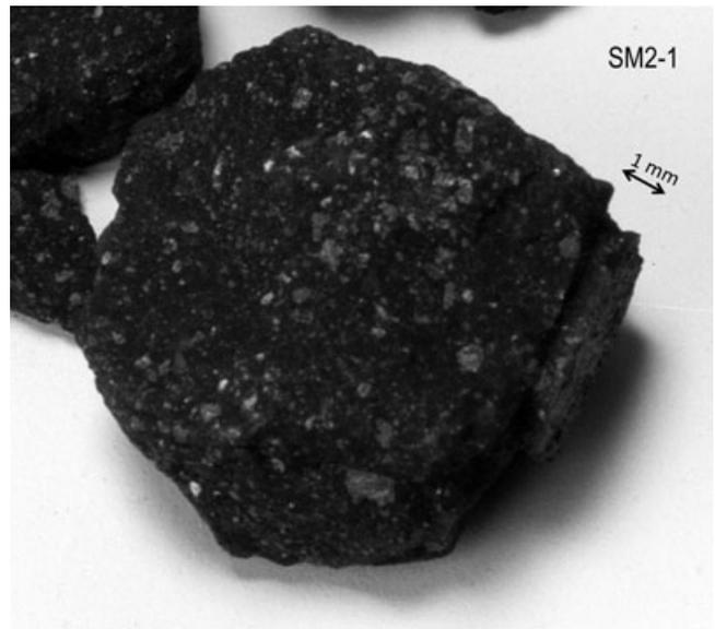
Fig. 1. Sutter’s Mill meteorite (individual SM2) that was used for this study (subfragment SM2-1d). Note that the fragment contained a piece of fusion crust almost 1 mm thick. (Double-headed arrow is a 1 mm scale bar.)
