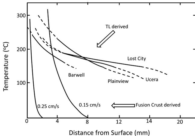
Fig. 4. Temperature gradients in meteorites caused by heating during atmospheric passage. The steep gradients at smallest distances into the meteorite are calculated from the thickness of various zones in the fusion crust, while the shallower gradients at larger distances are determined by thermoluminescence methods. (From Sears 1975.)
