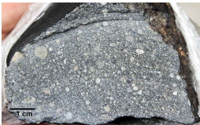
Fig. 1. Cut surface of the Vicência chondrite, showing abundant and beautifully developed chondrules and what appear to be chondrule, mineral and rock fragments, embedded into a gray to black, fine-grained matrix.
