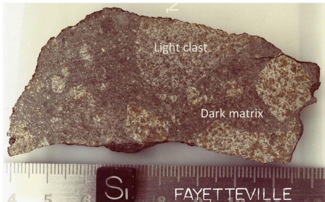
Fig. 10. A relatively small number of stony meteorites have a unique internal structure consisting of “normal” light clasts embedded in an unusual dark matrix which shows signs of being on the very surface of the asteroid. They are known as “gas-rich regolith breccias”. They are essentially true regolith that has been “lithified” by a shock sintering process which made it possible for them to come to Earth as meteorites. (From Schwarz and Sears, 1988).
